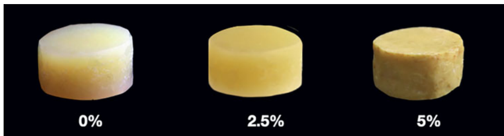
Fig 3 Cement specimens with \beta -AgVO 3 .
