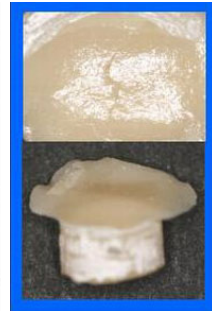
Fig.7 Specimen with cohesive fracture in the ceramic
