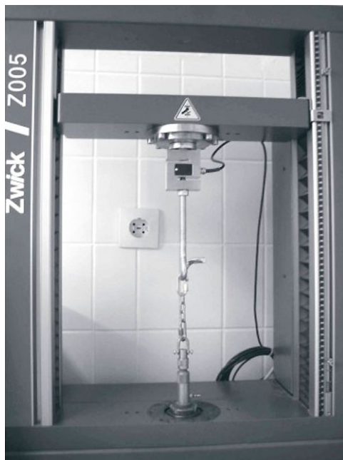
Fig. 4: Experimental device mounted in an universal testing machine (Zwick 005).
