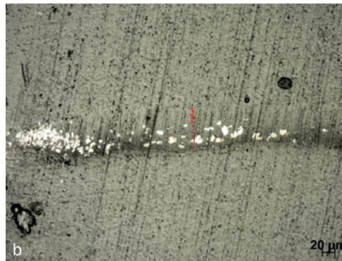
Fig 6 Representative image of leakage. a) Non-aged SbAd group showing few areas infiltrated by silver nitrate solution ( 4.67 \pm 2.87\% ) compared to b) non-aged Ad group showing greater infiltration by silver nitrate solution ( 12.85 \pm 1.70\% ).
