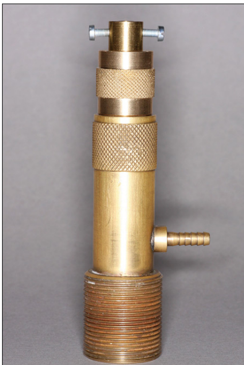
Fig. 5, 6: Special designed apparatus to test microtensile bond.
