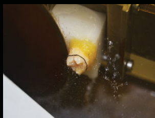
Fig. 1 – Dentin exposure with a diamond saw in a microtome
