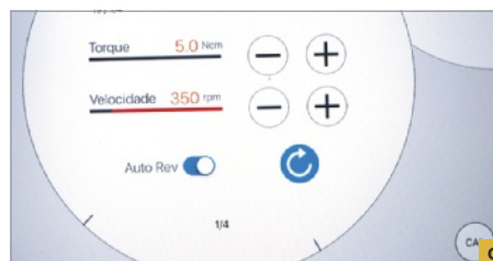
12C - Torque and speed programmed for the use of the bur. Bur used to remove the fiber post (Neodent Drill for Tempimplants, Ref: 103179; JJGC Ind e Comercio de Materiais Dentários SA, Curitiba, Brazil) coupled to the electric motor X-SMART IQ (Dentsply Maillefer).
