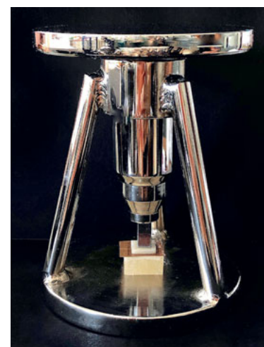
Fig 2 Special loading device that applies a 0.94 kg load to standardize pressure during cementation.
