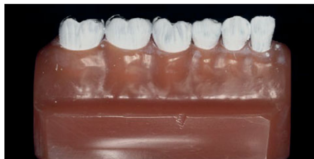
Fig 1 Experiment model, showing artificial teeth covered with a layer of titanium oxide.
