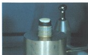
Fig. 1. Mounted dentin specimen on the perfused chamber.
