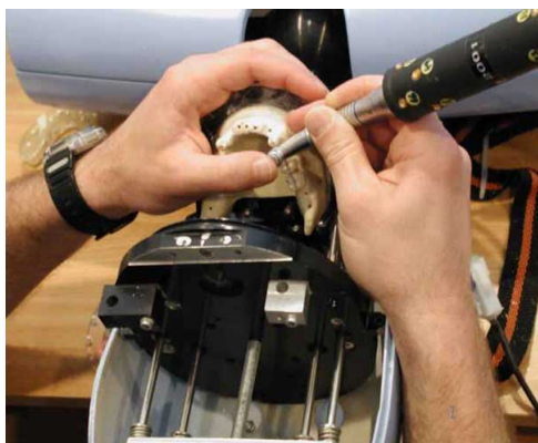
Executing the drilling, tracking the exact position of the handpiece and the patient (in fixed position).
