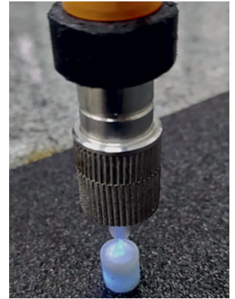
Fig 7 Light curing of a representative specimen with the optical fiber accessory tip through the hollow of the intraradicular post.
