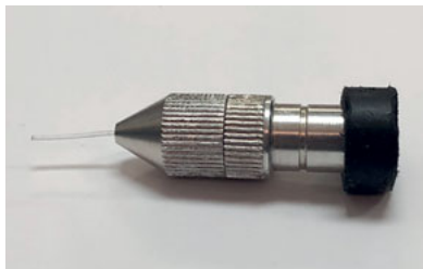
Fig 2 Accessory device in which the optical fiber is inserted and coupled to the light-curing unit.
