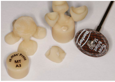
Figure 4 Removed and cleaned hot pressed restorations. Processing method: e.max Press (Ivoclar, Schaan, FL).
