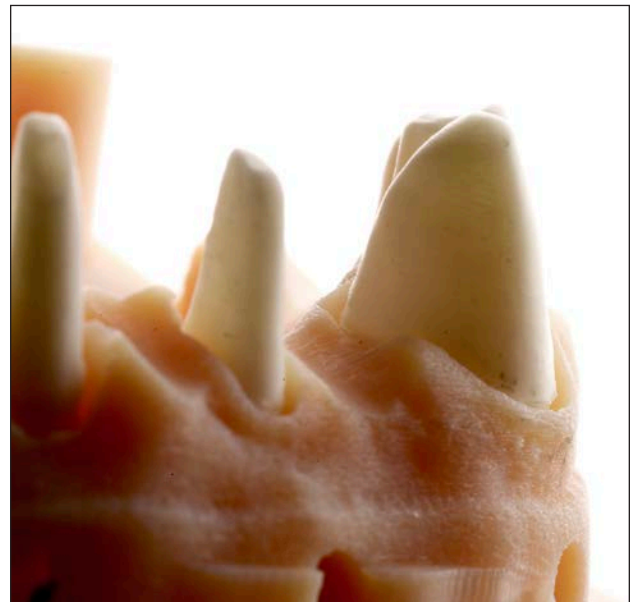
Fig 22 If the die is made in 10- \mu\text{m} layers, the demarcation between layers and tessellation are difficult to appreciate; thus, it can be used to manufacture restorations with either analog or digital techniques.
