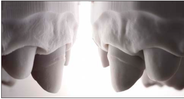
Fig 16 The quality of the model should not be judged by appearance. These two models were printed with the same DLP printing technology and 40- \mu\text{m} layers but with different resins and positioning in the printing vat. The model on the right appears truly uniform compared to the one on the left, but with a lower accuracy in replicating the intraoral scan file.
