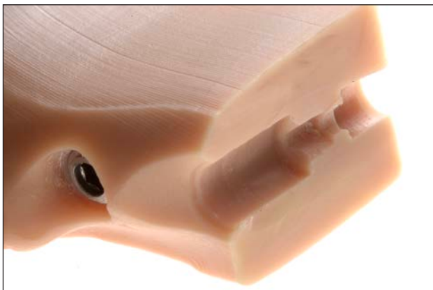
Fig 25 Cross-cut view of an implant analog housing. Due to their layered construction, 3D-printed models can replicate even complex shapes.
