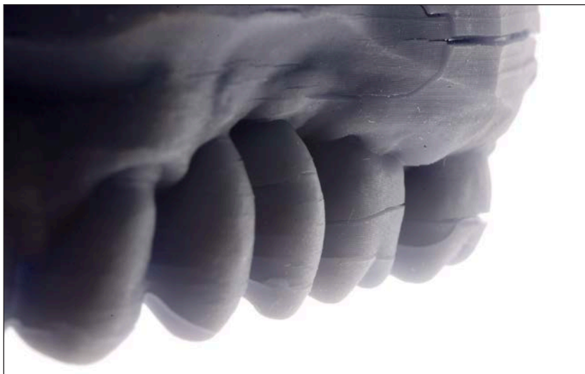
Fig 9 When the resin for 3D-printed models does not have an adequate flexural strength and flexural modulus, the tensions and deformations can cause cracks in their surface within a matter of days.
