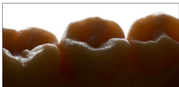
Fig 8 When the print layer has a height greater than the detail to be replicated, the print does not describe the object optimally, and islands of material are created (tessellation). This model was printed with 75- \mu\text{m} increments.
