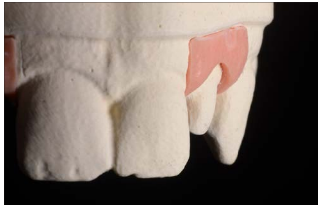
Fig 6 To achieve fast and economical milling, a soft type III plaster and an intermediate finishing grade have to be used. However, this model can easily chip.
