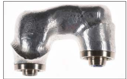
Fig 32 A milled aluminum jig can be created to verify the correspondence between the implant positions in the intraoral scan and the real position in the patient's mouth.
