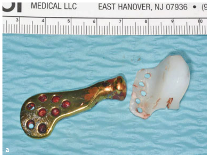
Figs 1a and b Explanted joint prosthesis (manufacturer and material unknown) with ramus and fossa component (a). The detailed view shows clear signs of wear in the synthetic fossa component and the metal condyle (b).
