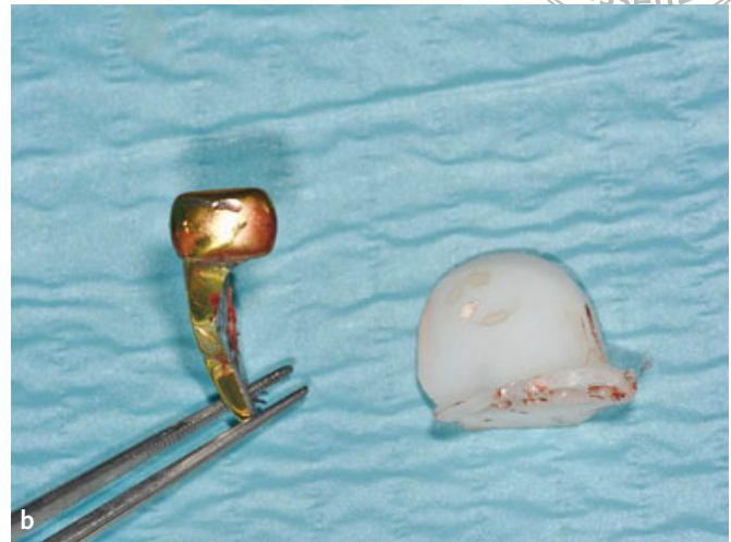
Figs 1a and b Explanted joint prosthesis (manufacturer and material unknown) with ramus and fossa component (a). The detailed view shows clear signs of wear in the synthetic fossa component and the metal condyle (b).
