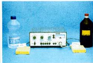
Figure 1: This figure shows the equipment necessary for iodine iontophoresis. It consists of a irritation current generator (Erbogalvan D2) and two sponges connected to the generator. The sponge connected to the negative pole (cathode) is moistened with the potassium iodide solution. The other sponge is connected to the positive pole (anode) and moistened with physiological saline.
