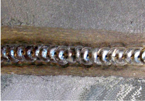
Fig. 3a: Craters on the welding surface associated with cracks along the welding rib: a. macroscopically aspect
