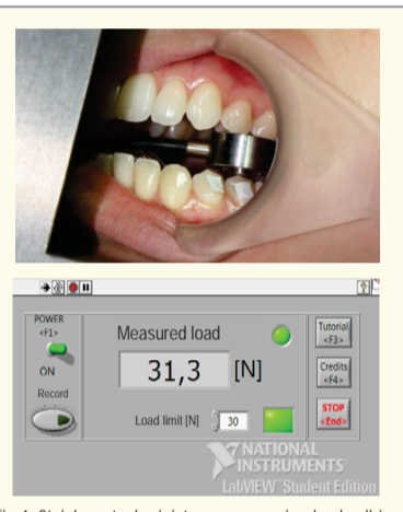
Fig 4. Stainless steel miniature compression load cell in position for images capture (Applied Measurements, Berkshire, UK) and correspondent Interface of the system design software LabVIEW 2010 (National Instruments®, Texas, USA) for measuring and recording the load bite application.
