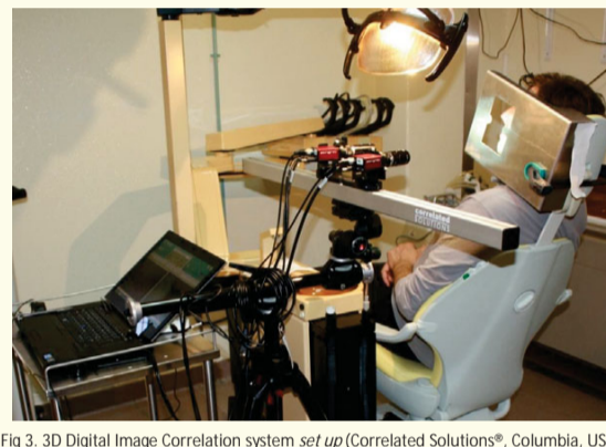
Fig 3. 3D Digital Image Correlation system set up (Correlated Solutions®, Columbia, USA).
