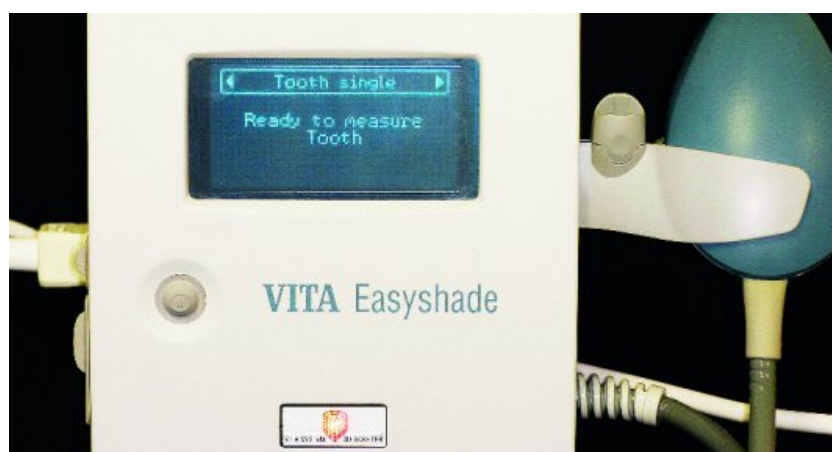
Abbildung 2 Vita Easyshade Dental-Spektrophotometer. Figure 2 Vita Easyshade Spectrophotometer.
