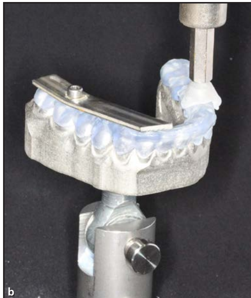
Fig 1 Experimental setup. (a) Cyclic pull-off testing chamber with splint, occlusal fixation, and vertical pull-off fixation. (b) Fracture test.
