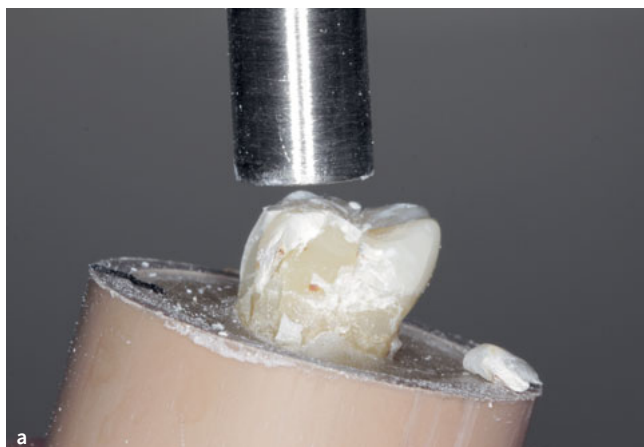
Fig 4a and b Sample mounted at 15-degree angle for fracture resistance test (a). Catastrophic fracture of the sample of 4 mm intracoronal depths after resistance load (b).
