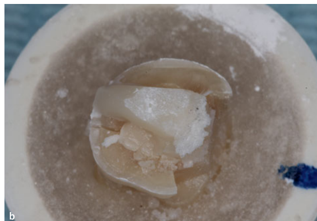
Fig 4a and b Sample mounted at 15-degree angle for fracture resistance test (a). Catastrophic fracture of the sample of 4 mm intracoronal depths after resistance load (b).
