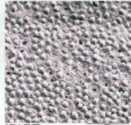
Fig. 6: Specimen loaded with 100 constant cycles before fracture. SEM, 2000x.
