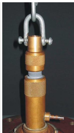
Fig. 2: Special designed apparatus mounted in the universal testing machine.
