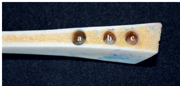
Fig 3 Bovine rib phantom used to evaluate the distance from the cortical bone. (a) 1 mm wear of cortical bone, (b) 1 mm from cortical bone and (c) 3 mm from cortical bone.
