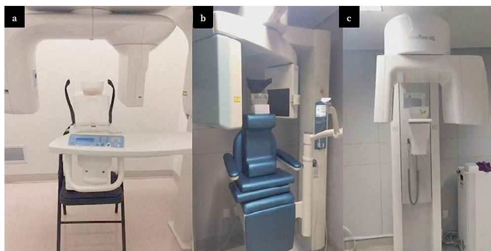
Fig 3 Scanning condition of the phantom. (a) CS 9300; (b) 3D Accuitomo; (c) Newtom VGi).
