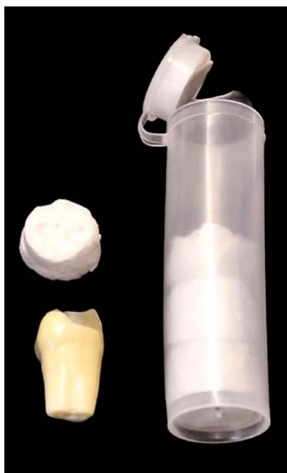
Fig 3 Each restoration was fixed on the tooth by wrapping a thin strip of adhesive tape around the pair. The samples were then placed in a plastic tube, and a light cushion was applied on top to prevent movement during the imaging. No cement layer was present; there was only an air layer between the tooth and restoration.
