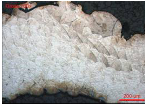
Fig. 4: Pile of the layers of Cr-Co
