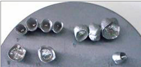
Fig. 7: Prosthetics restorations obtained by laser sintering
