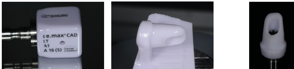
The abutment was milled out of a lithium disilicate block with an appropriate colour and fit-checking on corresponding titanium base was made before crystallization process of the glass-ceramic material.
