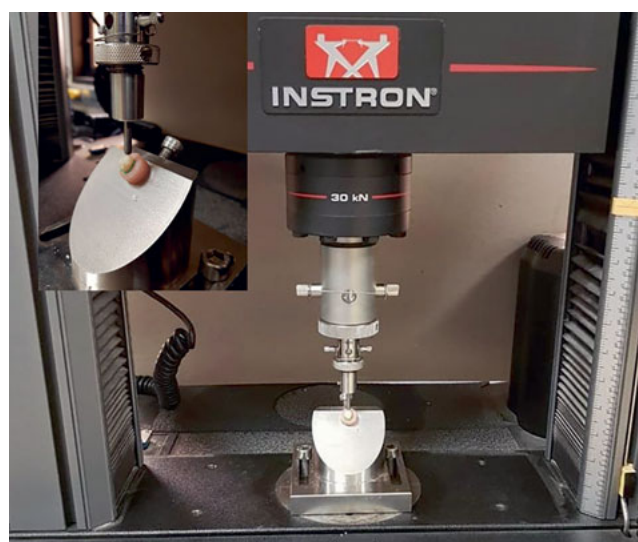
Fig 2 Compressive load testing set-up on the computer-controlled universal testing machine (Instron 8967).
