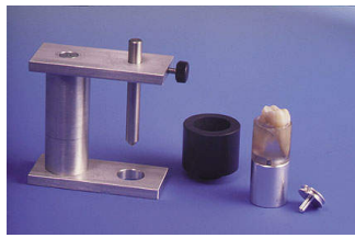
Fig 1a - Experimental setup: Tomography scanner left and Open VMS machine Fig 1b - Alignment tool, mould and specimen holder Fig 2 - Instruments tested in this study: GT-Files, NiTi K Files, Lightspeed and ProFile .04 Dentsply-Maillefer, Ballaigues, CH & Lightspeed Inc, San Antonio TX, USA (from left to right).
