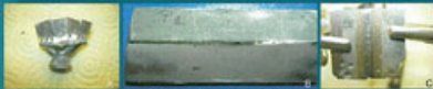
Fig. 2. Different welding types: A. Cast plates; B. Laser welding; C. Micropulse welding.
