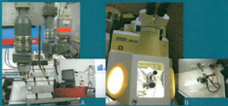
Fig. 1. Welding equipments: A. Nd:YAG laser - HL 124P LCU TRUMPF; B. micropulse Welder.
