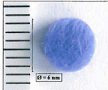
Figure 2: Non woven scaffold made of PGA
