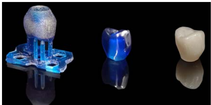
Figure 7 Example of a 3D printing process (V-Print Cast, Voco, Cuxhaven, D) for the production of a pressed lithium (di)silicate crown. Left image: printed object in light-cured state after CAD production. Middle picture: fitted and finished resin crown before investment. Right image: finished ceramic crown.
